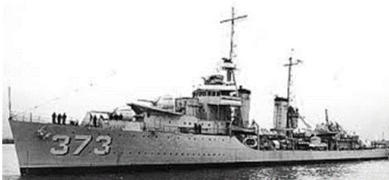
The USS Shaw had been commissioned only 5 years before and was capable of a maximum speed of 35 knots. It was armed with 4x5 inch guns, 12x21 inch torpedo tubes, 4 Bofors 40 mm AA (2x2), 6x20 mm AA, 2 depth charge roll-off racks and 4 K-gun depth charge projectors. For its day, the Shaw was a well-armed naval vessel. All naval personnel had an assigned battle station. Even as a Ships' Cook, Anthony would have had his place at one of the firing positions.
