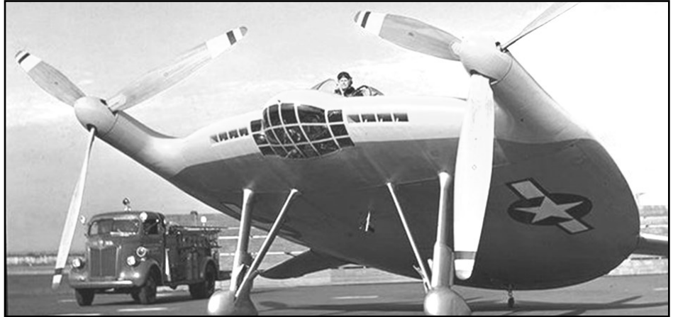
The Vought V-173 "Flying Pancake" was an American experimental test aircraft built as part of the Vought XF5U program during World War II
